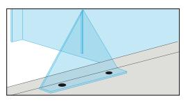
SIDE SCREEN OPTION: SCREWED FROM THE UNDERSIDE OF THE DESK TOP IF THE SCREEN NEEDS TO BE SECURED MORE FIRMLY.
